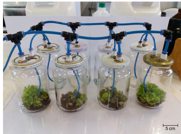
Figure 1: Bioreactor with dual container system (500 mL capacity).
