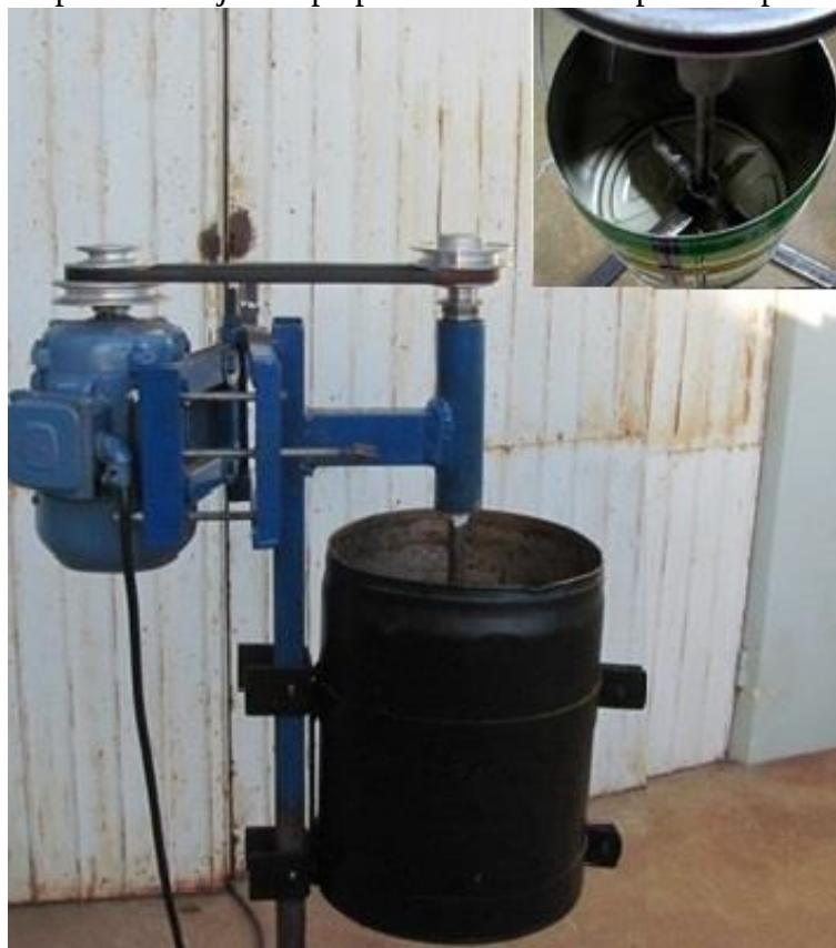
Figure 2. Pulper developed for the jerivá pulp and seed initial separation process
